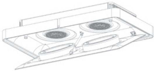
Open the bottom panel by pulling it open on the front side with 2 hands in a downward movement.
